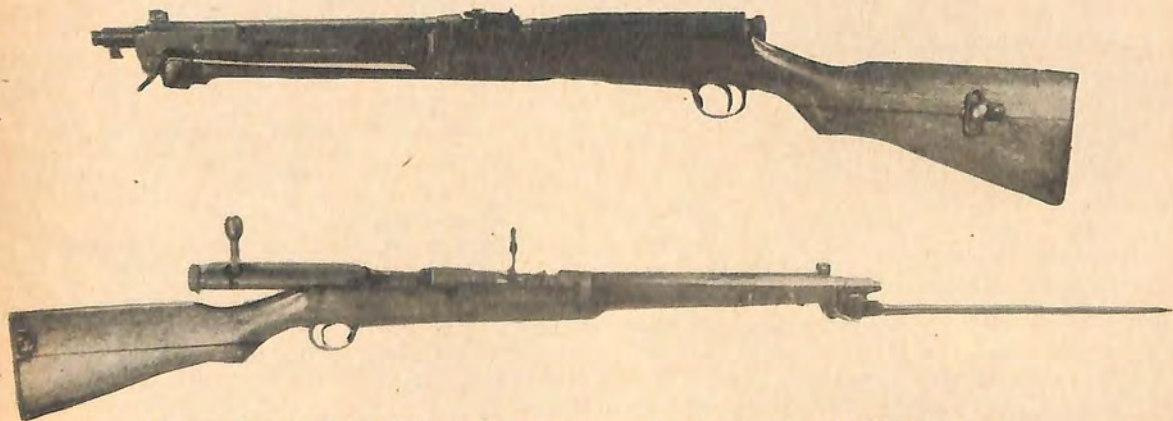
Figure 172. Model 44 (1911) 6.5-mm cavalry carbine (showing bayonet folded and open).
